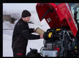
The well proportioned cooling package is easy to access, clean and maintain. The engine air filter is also very easy to access
