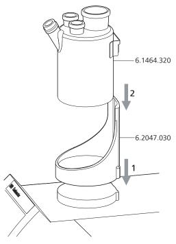
Figure 3 Inserting the titration cell (coulometry)
