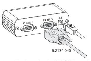
Figure 29 Connecting the RS-232/USB Box to the PC
