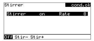
The stirring rate can be reduced with **Stir-** and increased with **Stir+**. **Off** switches the stirrer off. **On** is now displayed instead. This can be used to switch the stirrer back on. This dialog is exited with **[BACK]**.
