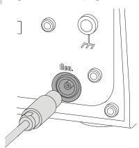
Figure 11 Connecting a generator electrode
