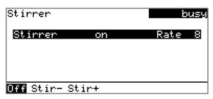
The stirring rate can be reduced with **Stir-** and increased with **Stir+**. **Off** switches the stirrer off. **On** is now displayed instead. This can be used to switch the stirrer back on. This dialog is exited with **[BACK]**.
