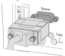
Figure 22 Connecting a remote cable
