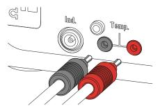
Figure 15 Connecting a temperature sensor
