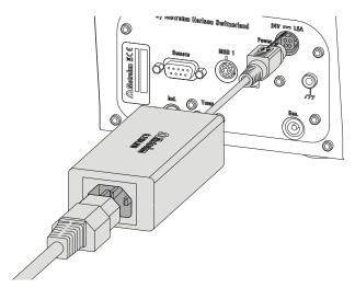
Figure 7 Connecting the power supply unit
