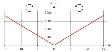
Figure 25 Rotational speed depending on the stirring rate
