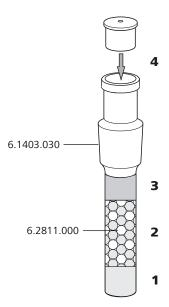
Figure 4 Filling the adsorber tube
