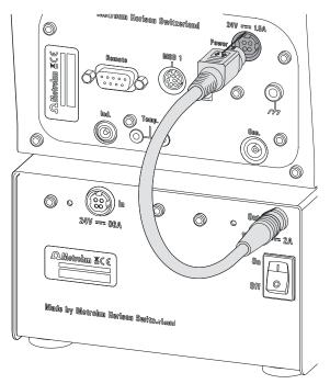
Figure 8 Connecting the Power Box
