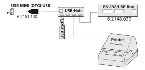
Figure 21 Connecting the USB hub with USB flash drive, printer and 6.2148.030 RS-232/USB Box
