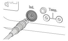
Figure 14 Connecting an indicator electrode
