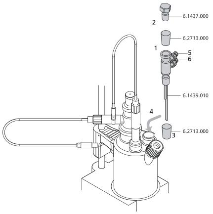
Figure 6 Mounting the addition and aspiration tube
