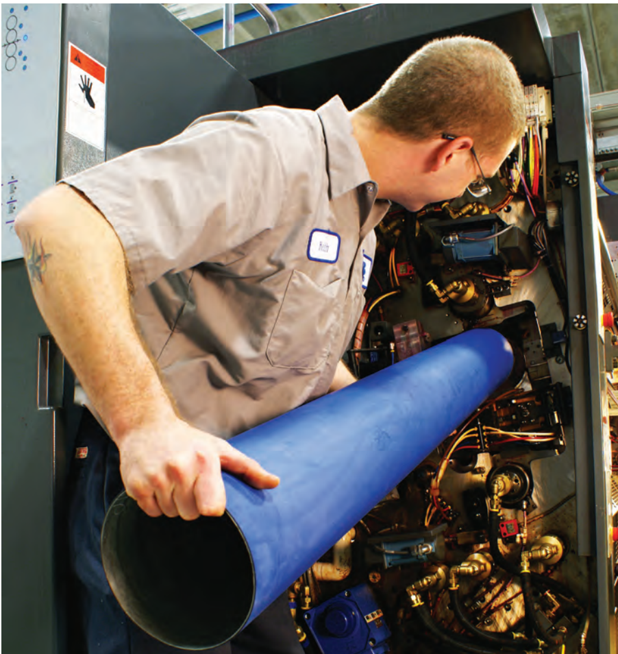
Gapless blankets slide in through the side frame and can be changed in less than one minute without removing the web.
